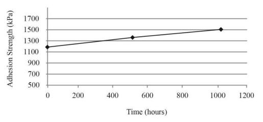
DOWSIL SE 1720 CV Adhesive Adhesion Strength Over Time during  $85^{\circ}$ C/ $85^{\circ}$  RH Exposure
