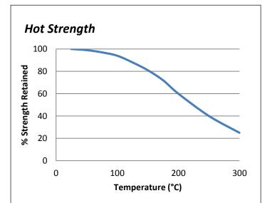
"Hot strength" shear strength tests performed on mild steel. Fully cured then conditioned to pull temperature for 30 minutes before testing. ES5505 can withstand higher temperatures for brief periods (such as for paint baking and wave soldering processes) providing the joint is not unduly stressed. The minimum temperature the cured adhesive can be exposed to is -40°C (-40°F) depending on the materials being bonded.
